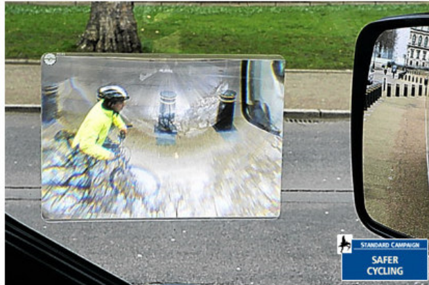
Breakthrough: a Fresnel lens fixed to the window of a lorry cab
